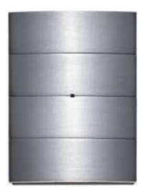
The application module for pushing onto the flush-mounting bus coupling unit. Depending on the user software can trigger switch actuators, or dim actuators or shutter actuators, and can also be used as a value transmitter for transmitting brightness values, or for extension operations of the light scene push button.
